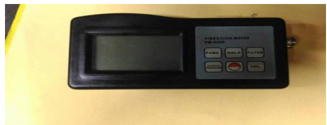
Figure no. 6 : Vibration meter
