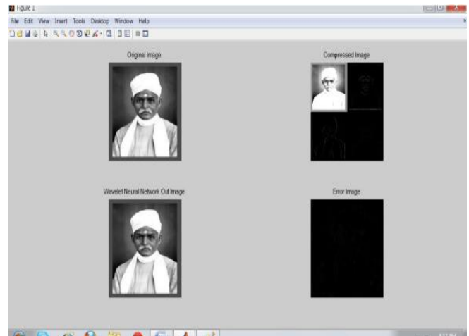
Figure 9: Image compressions by MLP with wavelet coefficients (25% compression)
