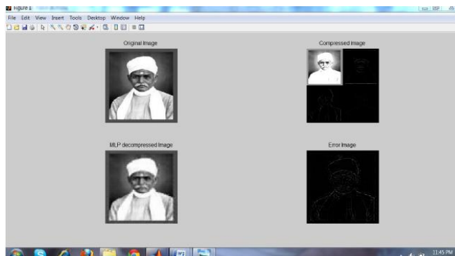
Figure 15: Image by MLP with wavelet coefficients (87.5% compression)
