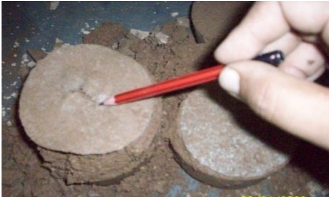
Plate.3. Rupture failure of fabric reinforcement
