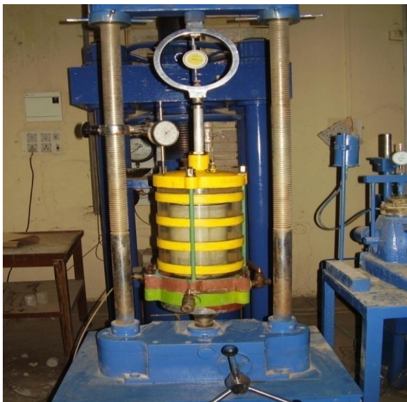
Plate 2. Large triaxial test–Experimental set up
