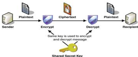
Figure 2.1: Diagram illustrating symmetric encryption.
