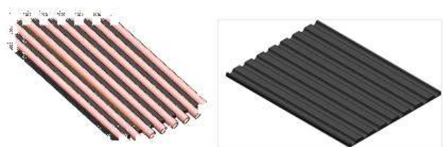
Figure 5.3 surface contact area of absorber plat and collector riser pipes in the grooved part
