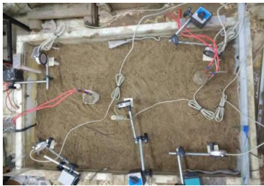
Figure 1. Sketch map of settlement monitoring arrangement
