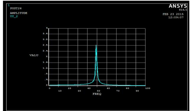
**Fig 5.** Frequency Vs Displacement plot for Steel
