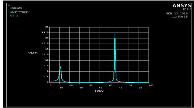
**Fig 4.** Frequency Vs Displacement plot for Lead
