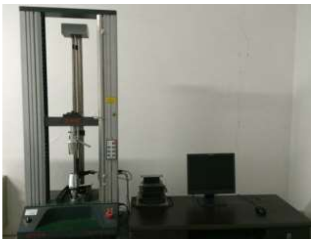
Fig. 1 Material testing machine controlled by computer
