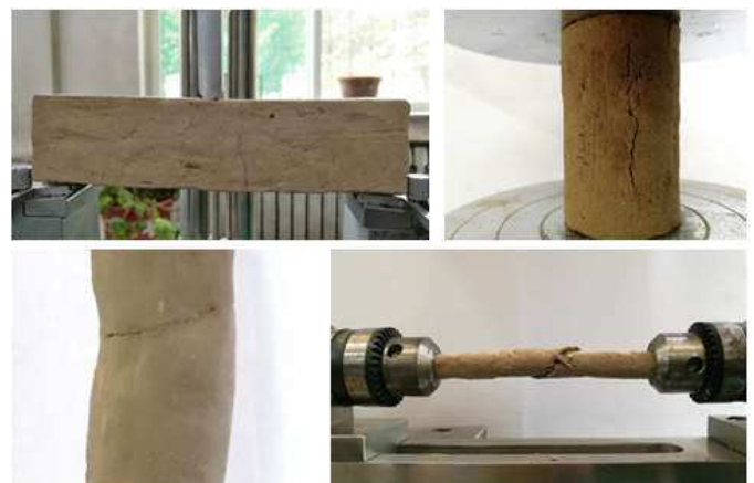
Fig.4 Surface cracks of specimens (including bending, compressive, bending and tensile and torsional strength tests) Excel software is used to calculate the mean value of repeated samples with limit values. The results are summarized as table 3:
