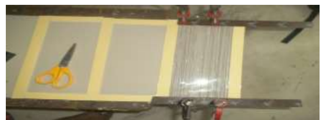
Fig.2.2.2(c) Composite at curing
