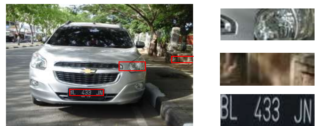
Figure 10. In the left side image shows that the candidate plates have been obtained, and in the right side images show the cropped plate candidates.
