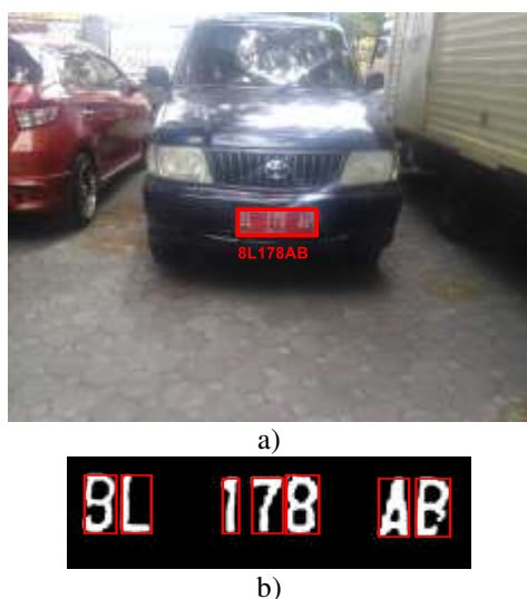
Figure 15. a) Misclassification of Q Character b) The result of characters segmentation. It is clearly can be seen that the result of character segmentation is not perfect. The Q character truncated at the bottom.
