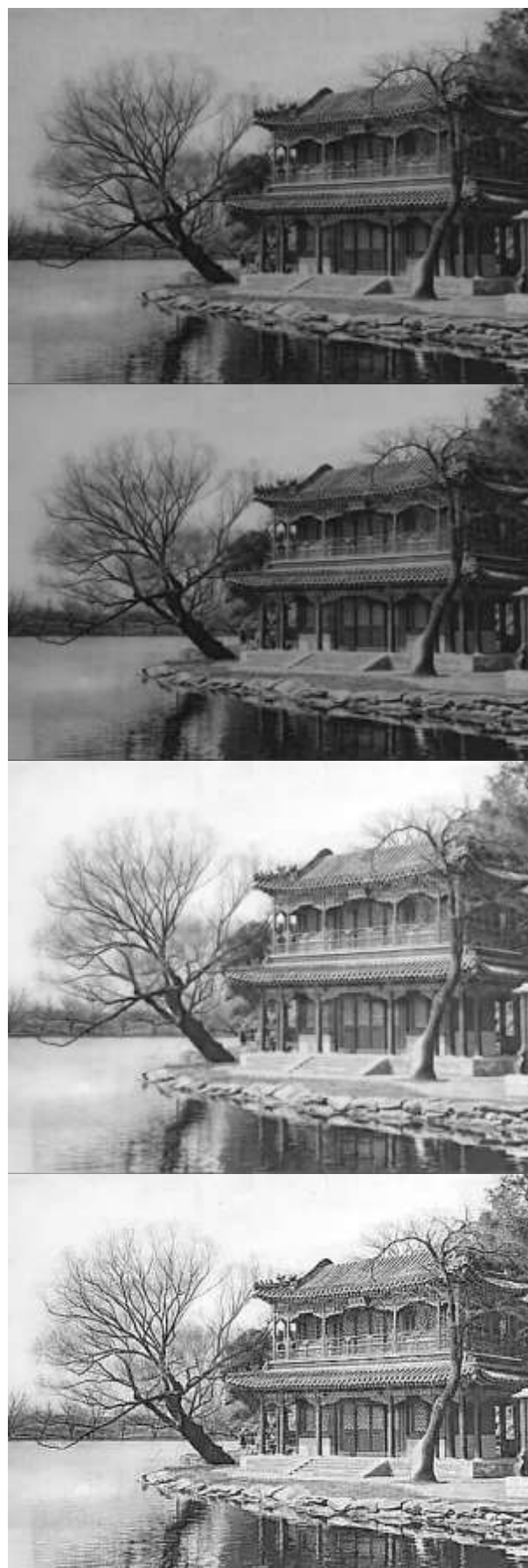
Fig. 3 Digital enhancement of an old building (from top-left to bottom-right). Original image, results through three steps in sequence: nonlocal means filter, adjustment of gray levels and unsharp mask filter, respectively
