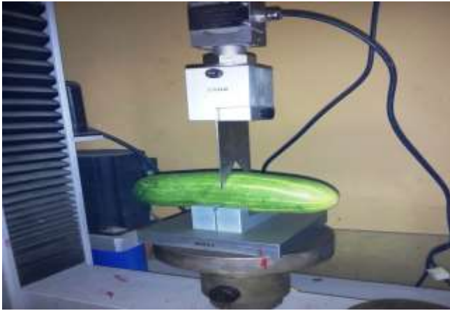
Figure 2: Cucumber fruit undergoing Warner Bratzler Test, using Universal Testing Machine (Testometric model, series 500-532)
