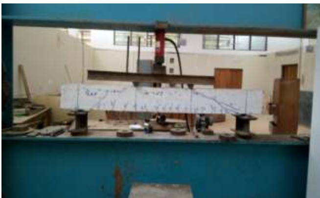
Fig. 7. F-series beams failed in diagonal shear predominantly
