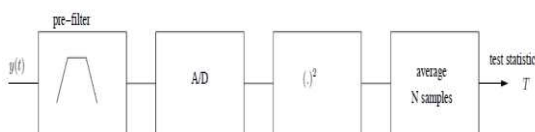
Figure 7: Block diagram of an Energy Detector. [26]
