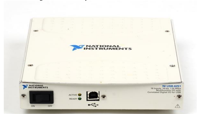
Fig. 4.10. DAQ card NI USB - 6251 used for experiment [19]
