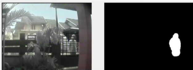
Fig. 4. Color image and background subtracted for example of normal activity
