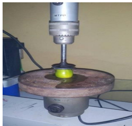
Figure 2: Gmelina fruit undergoing compression testing (Axial loading orientation)
