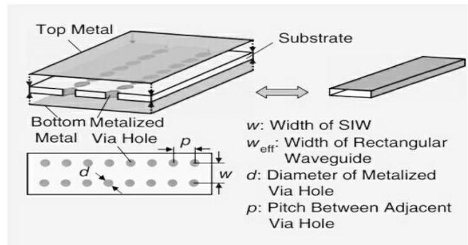
Figure 3: An SIW and its equivalent rectangular waveguide [2].
