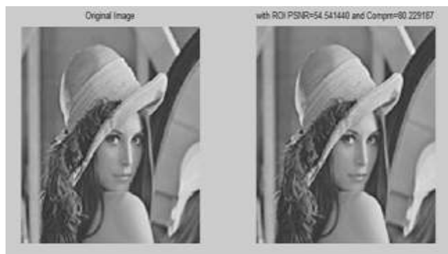
Figure 9 Original Image and With ROI PSNR=54.541440 and Comprn=80.229187
