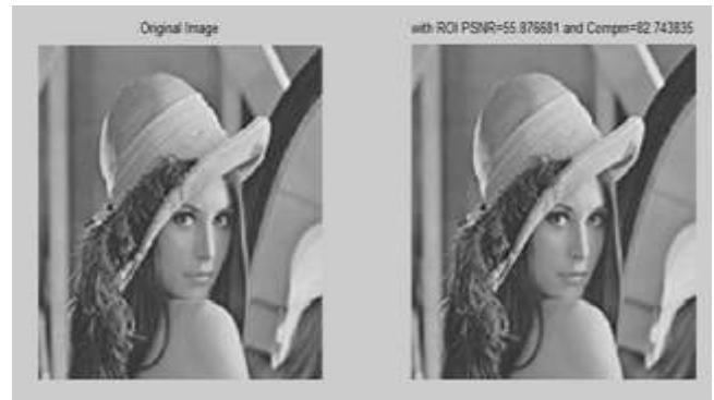
Figure 10 Original Image and With ROI PSNR=55.876681 and Comprn=82.743835
