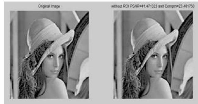
Figure 16 Original Image and Without ROI PSNR=41.471323 and Comprn=23.481750
