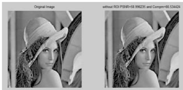
Figure 20 Original Image and Without ROI PSNR=58.996235 and Comprn=66.534424
