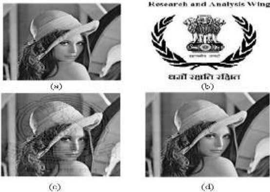
Figure 2: (a) the original Lena image (b) logo to be watermarked (c) visible watermarked image and (d) invisible watermarked image.
