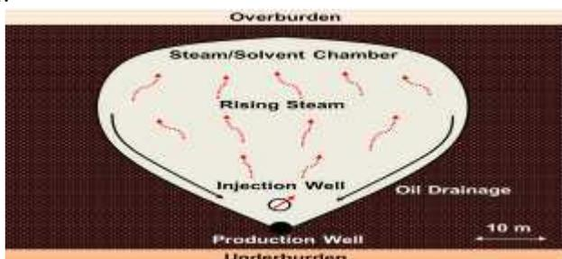
Fig. 1 Concept diagram of SAGD and solvent-SAGD process.
