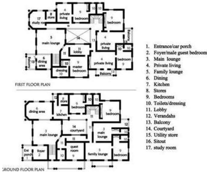
Figure 9. Plan of a Contemporary Hausa Building Designed by Zailani and Sa'ad Raji (Aliyu, 2015).
