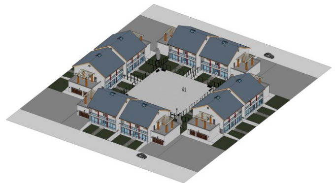
Figure 26. Beijing new courtyard garden house compound based on a system of 78 m × 78 m standard block size, the communal courtyard is 26 m × 26 m shared by eight nuclear families, with each household enjoying a private garden of 12 m × 6 m at the front and the back. Each housing unit measures 10 m × 12 m (total 240 sqm) with a semi-basement and 2 ½ storeys. Design and computer model by Donia Zhang 2015c, 2016b.
