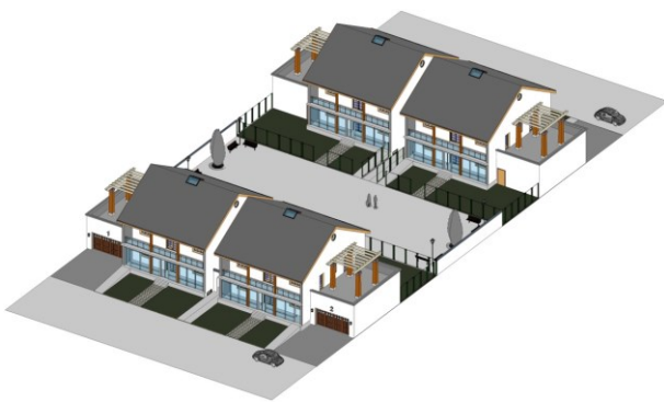
Figure 28. Suzhou new courtyard garden house compound based on a system of 40 m × 66 m standard block size, the communal courtyard is 14 m × 40 m shared by four nuclear families, with each household enjoying a private garden of 12 m × 6 m at the front and the back. Each housing unit measures 10 m × 12 m (total 240 sqm) with a semi-basement and 2 ½ storeys. Design and computer model by Donia Zhang 2015c, 2016b.
