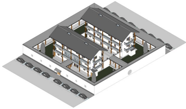
Figure 27. Suzhou new courtyard garden house compound based on a system of 40 m × 40 m standard block size, the communal courtyard is 12 m × 20 m shared by four nuclear families, with each household enjoying a private garden on the side. Each housing unit measures 6 m × 10 m (total 180 sqm) with 3 storeys. Design and computer model by Donia Zhang 2016b.
