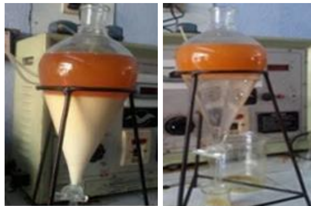
Fig. 4 Soaps separation Fig. 5 Clean water in washing
