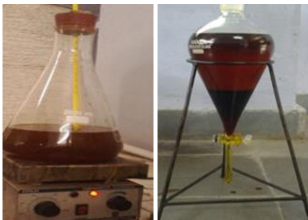
Fig.2 Acid treatment Fig. 3 Glycerin separation
