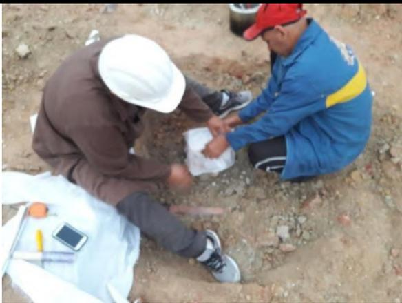
Fig. 2: Undisturbed block of soil
