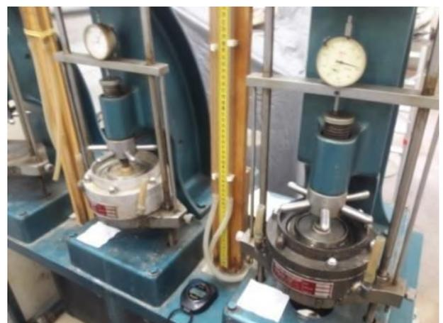
Fig. 4: Oedometric Test
