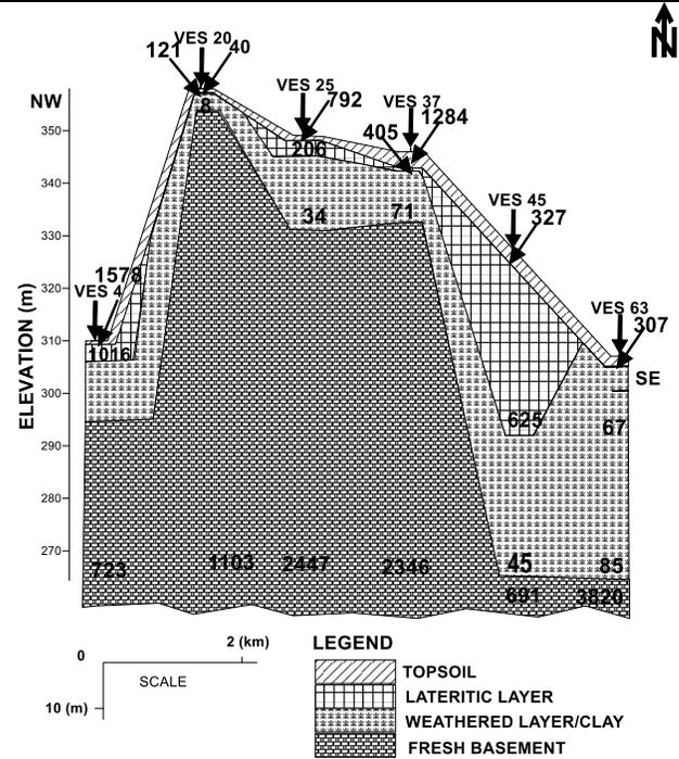
Fig.5b: Geoelectric Section along NW-SE
