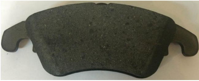
Fig.2: The new semi – metallic brake pad.
