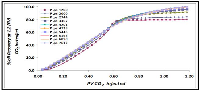
Figure (25): Results of displacement test for sample NO. (2)
