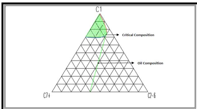
Figure (3): Ternary phase diagram for a hydrocarbon system: the limiting tie line passes through the oil composition at minimum miscibility pressure (MMP).
