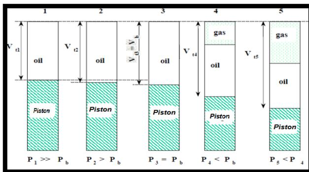
Figure (5): Constant mass depletion test.
