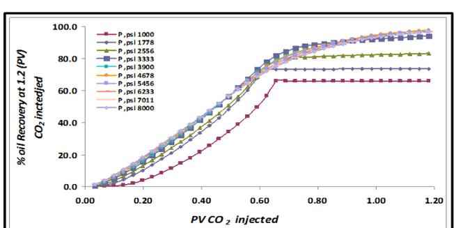
Figure (29): Results of displacement test for sample NO. (5)
