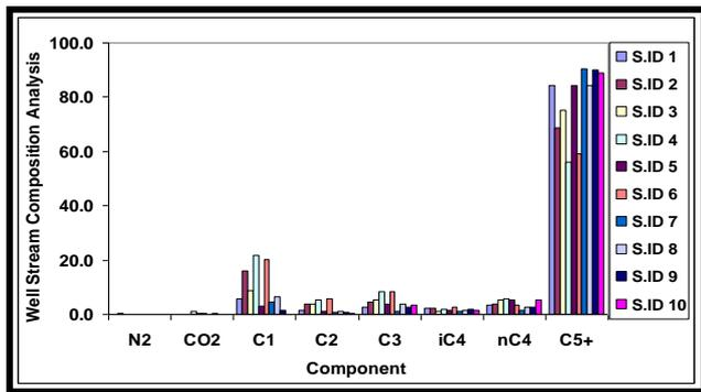
Figure (13): Variation of reservoir fluid composition analysis for ten Egyptian live crude oils
