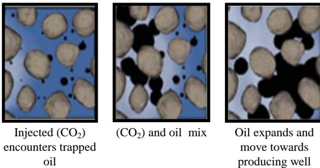
Figure (2): The following photographs illustrate (CO<sub>2</sub>) miscible process for oil reservoir.
