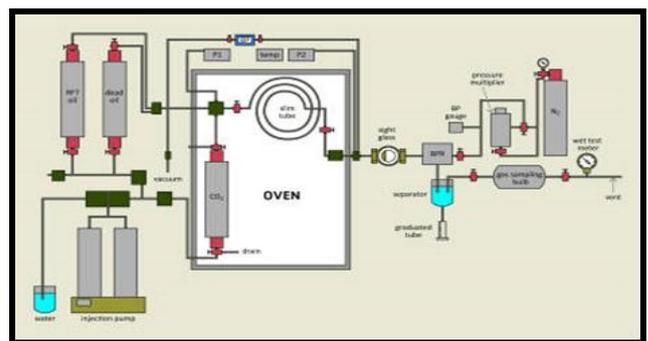
Figure (6):Schematic of slim tube setup
