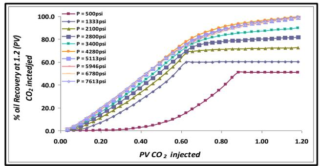
Figure (24): Results of displacement test for sample NO. (1)
