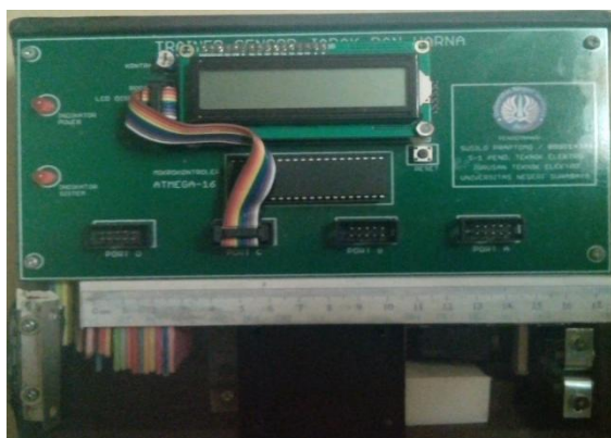
Figure 3. Trainer Sensor distance and color sensor
