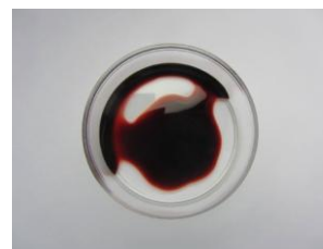
Figure 1. Photograph of a typical used dyeing liquor consisting of an IL and the dissolved disperse dyestuff.
