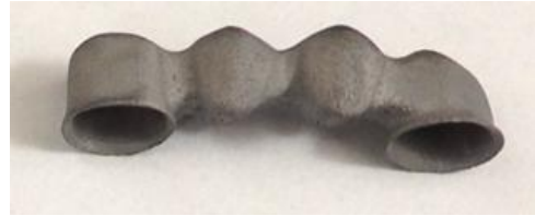
Fig. 3. View of prosthetic foundation after sand-blasting
