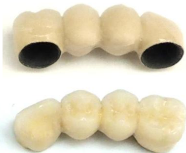
Fig. 6. View of the ready-to-use prosthetic bridge made of Ti-13Zr-Nb with ceramic coating
