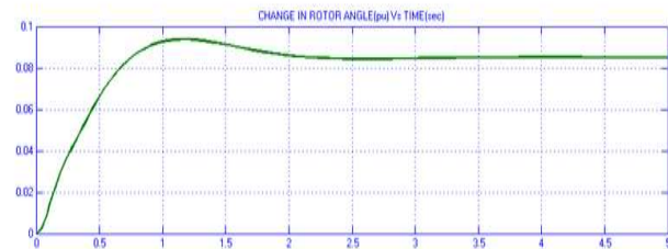
Fig.5. change in rotor angle of the rotor of SMIB with PSS (PID-ZN method)
