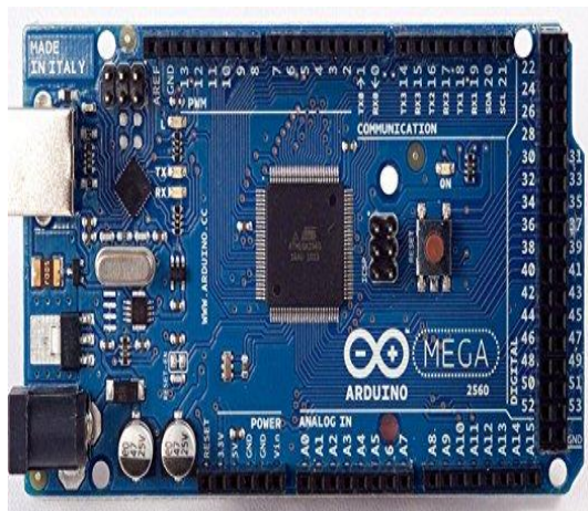
Fig 2. General Structure of Arduino ATmega2560 development board
