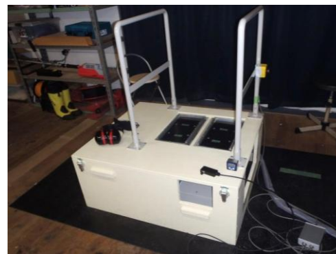
Figure. 1 A new device for measuring proprioceptive sense of the ankle joint
