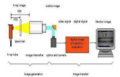
RTR inspection is especially applied for the casting materials, which are produced for automotive, and airplane industry, acceptable defect type and defect size is so a few. Real time radioscopic method has been developed for the last few years and it is widely used in Al wheel production lines.
