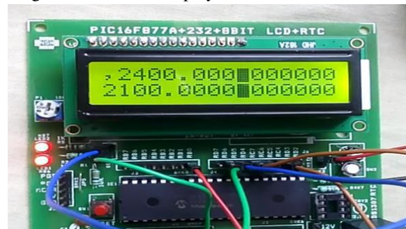
Fig : 8 Display of boundary values (before calibration)
