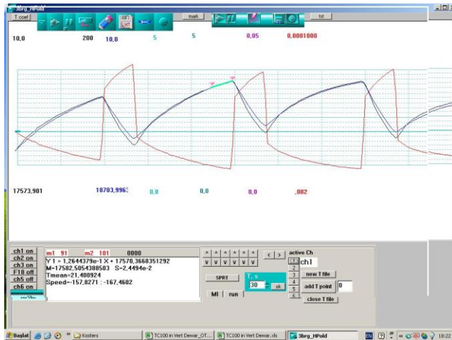
Fig.2. Simultaneous records of the resistance variations of a platinum resistance thermometer (PRT) and of two thermistors Th-1 and Th-2, which are located symmetrically relative to the PRT on the surface of the gauge block. During the current modulation cycle in the PRT, its current for 1/4 of the modulation period is kept at the level of 5\text{mA} and 3/4 of the period is kept at 1\text{mA} . The sensitivities of the thermistors are, practically, equal. Two cursors (shown by triangles) define the averaging time for the mean values of temperature quantities. (See text for other details).
