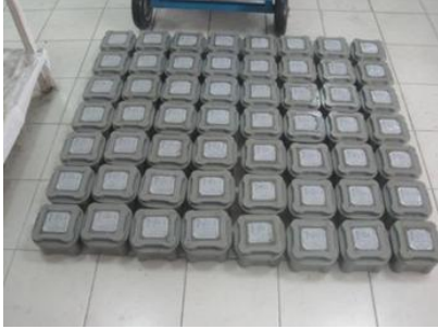
Fig.8. Concrete products with using C&D waste additive cement
