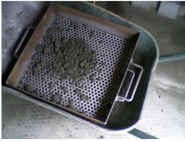
Fig.7. Clinker produced with using C&D waste addition
