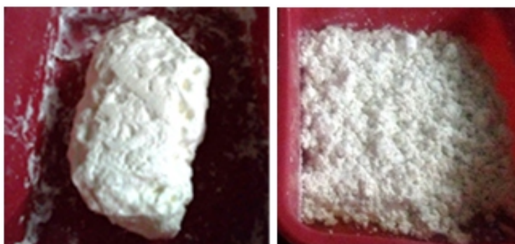
Gambar 1. Koagulum karet alam terhidrogenasi berpenstabil NaOH (kiri) dan SLS (kanan) Figure 1. Hydrogenated natural rubber coagulum, stabilized with NaOH (left) and SLS (right)
