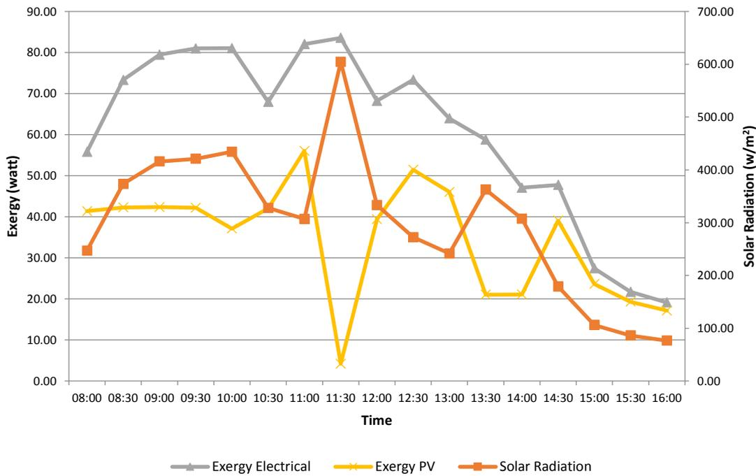
Figure 4. The relationship between solar radiation, electrical exergy, and exergy photovoltaic
