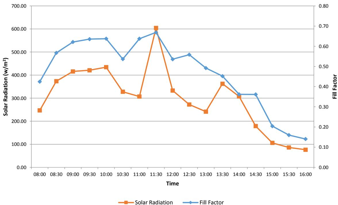
Figure 3. Effect of solar radiation on fill factor
