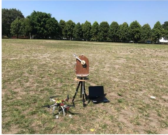
Figure 7. Antenna tracker performance test
