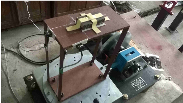
Fig. 6: Steel frame model 1 with extra mass at the center
