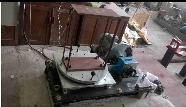
Fig. 5: Steel frame model 1 without any extra mass
