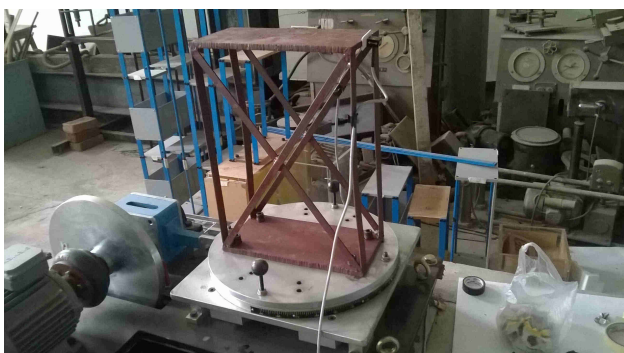
Fig. 8: Steel frame model 2 without any extra mass
