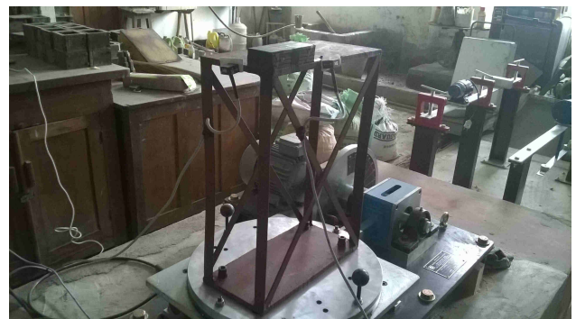
Fig. 10: Steel frame model 2 with extra mass at the corner
