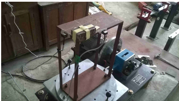
Fig. 7: Steel frame model 1 with extra mass at the corner
