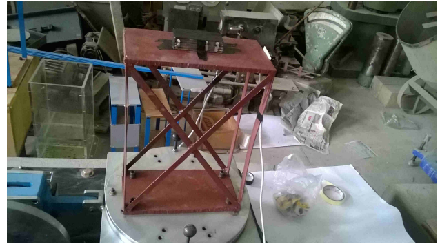
Fig. 9: Steel frame model 2 with extra mass at the center
