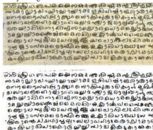
Fig.10: Original image (top) and the output of the spatial change detector (bottom)
