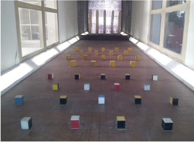
Fig. 1. Flow roughening devices placed inside the wind tunnel.
