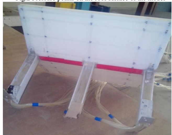
Fig.3 Perspex sheet model of Trough canopy roof
