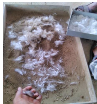
Fig. 3 Mixing of fiber and soil
