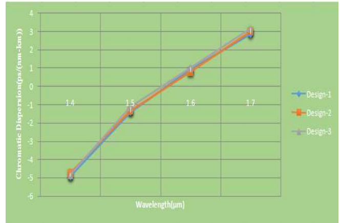
Fig. 6 Comparison of Chromatic dispersion for Design-1 to Design-3
