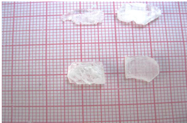
Fig. 1. Photograph of the grown \text{KSbF}_4 crystal
