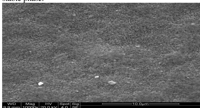
Figure 3. SEM image of TiO 2 thin film
