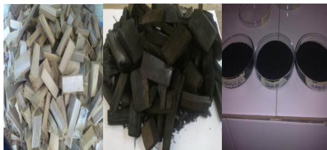
Fig 1 Pieces of Nigerian waste bamboo before, after carbonization and after activation.
